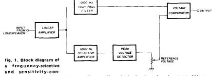
trolled ssty preamplifier which permits reception of ssty signals under adverse conditions.
